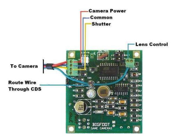
Note that there must be a diode connected from battery negative to the second common. JP2 should be jumped and JP1 should not.
